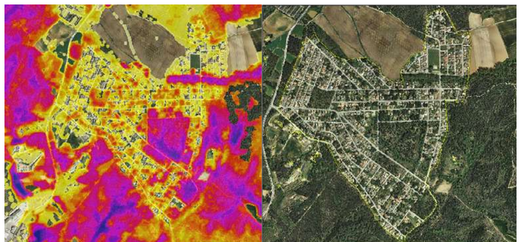
Radiation mapping of a WUI area for the identification of the working zones within it based on specific irrigation parameters.
